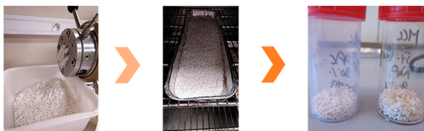
Figure 1. Extrusion-spheronization techniques with pine essential oil ( \alpha -pinene 26% and limonene 19%) [95].
