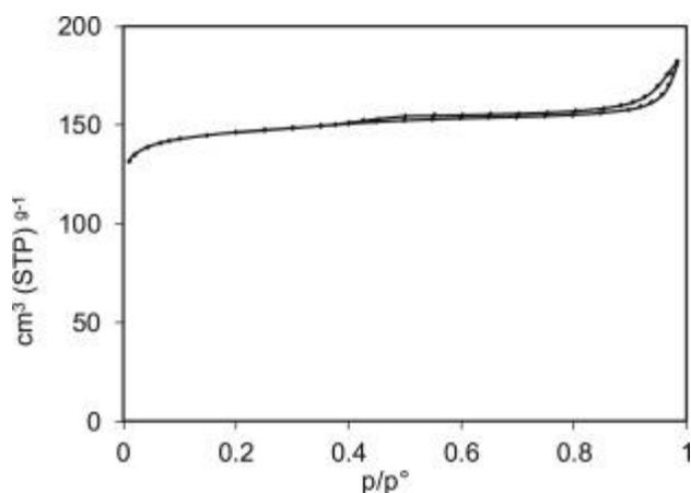
Fig. 2. Adsorption-desorption N<sub>2</sub> isotherm at 77 K.
