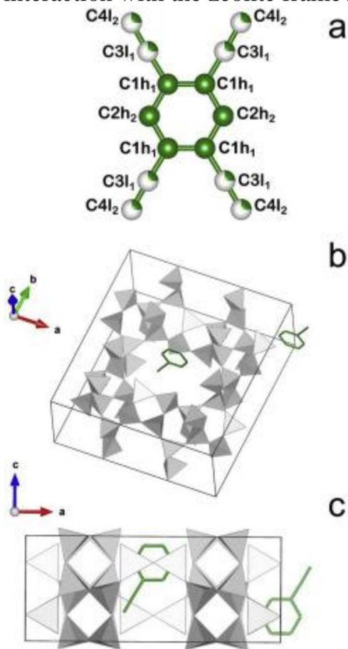
Fig. 4. a) Phenylacetylene molecule showing the labels used for the carbon sites. b) and c) Structural model of HS-MOR compressed in phenylacetylene at 0.40 GPa (H<sub>2</sub>O molecules are omitted for clarity). The two figures show only the average positions actually occupied rather than all the partially occupied symmetrically equivalent positions.
