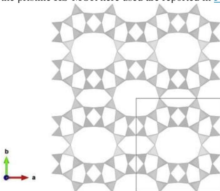
Fig. 1. MOR framework structure viewed along the [001] direction. Unit cell is drawn. Table 1. Data relative to the pristine HS-MOR used for phenylacetylene loading. \*taken from the structural refinement reported in Ref. [23].
