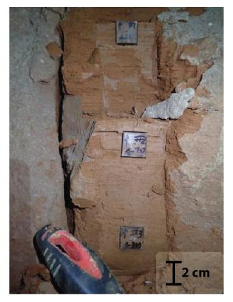
**Figure 4.** Example of clay sampling for the paleomagnetic study. Location at the entrance shaft (highest elevation of every samples,  $\sim 580 \, \text{m}$  a.s.l.; Leicasse cave system, Site 2, Fig. 1).
