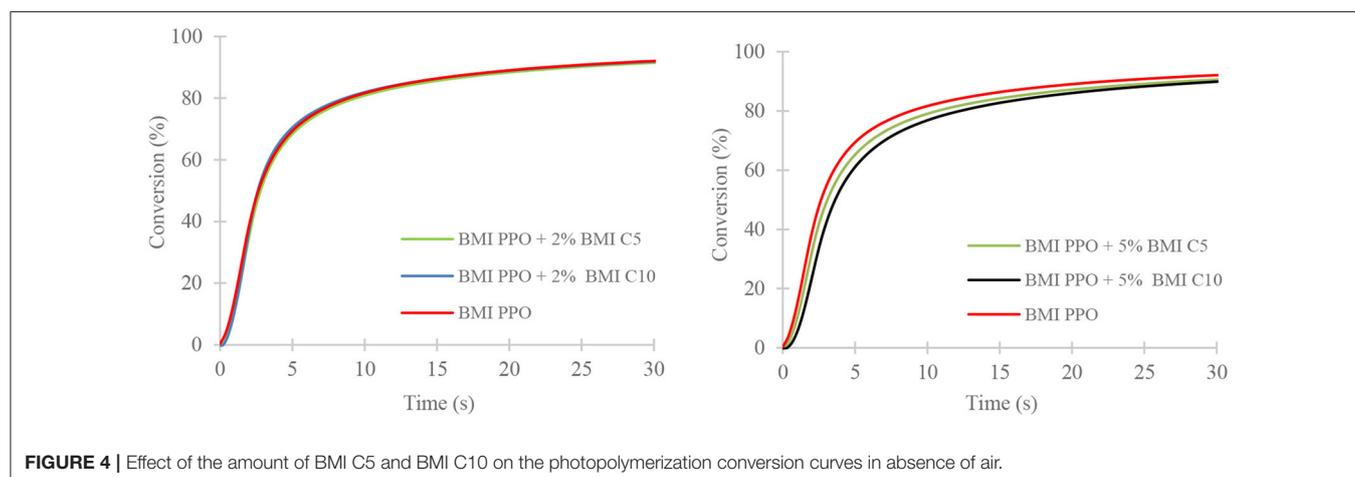
**FIGURE 4** | Effect of the amount of BMI C5 and BMI C10 on the photopolymerization conversion curves in absence of air.
