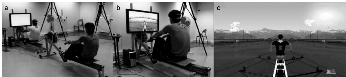
Figure 1. Experimental setup. (a) Coordination with the real teammate in the transfer condition. (b) Coordination with the virtual teammate in the other conditions. (c) Virtual environment displayed on the monitor.
