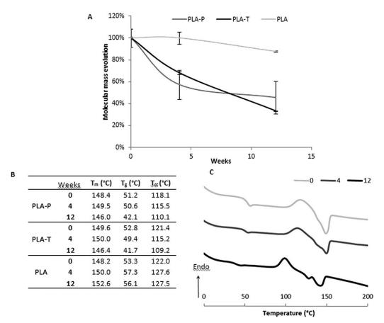
**FIGURE 5.** PLA-P, PLA-T and PLA degradation after 4 and 12 weeks of subcutaneous implantation: copolymers molecular weight evolution (A), mains copolymers thermal properties evolution (B) and illustration of PLA-P thermal properties evolution. Melting temperature ( $T_m$ ), melting enthalpy ( $\Delta H_m$ ), glass transition temperature ( $T_a$ ), and cold crystallization temperature ( $T_c$ ) determined by DCS.
