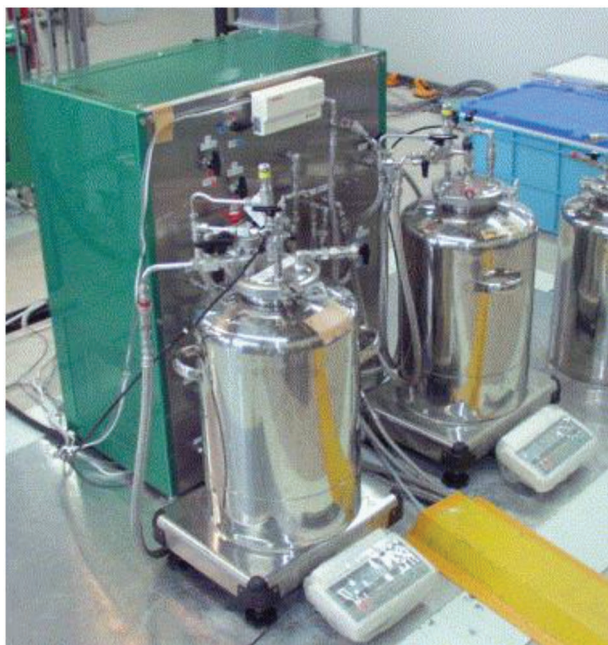
Figure 27. The hydrogen generator based on \text{NaBH}_4 developed by Kojima et al. [374] The two stainless steel tanks used to store the fuel (alkaline aqueous solution of \text{NaBH}_4 , 8.8 mol \text{L}^{-1} ) and the spent fuel (borates in aqueous solution) are shown. The system has a body size of about 200 L and a weight of 80 kg. With this prototype, the effective hydrogen storage capacities would be at best of 2 mass% \text{H}_2 and 15 kg ( \text{H}_2 ) \text{m}^{-3} , which would be comparable to a compressed \text{H}_2 system at 25 MPa. Reproduced with permission. [374] Copyright 2004, Elsevier B.V.
