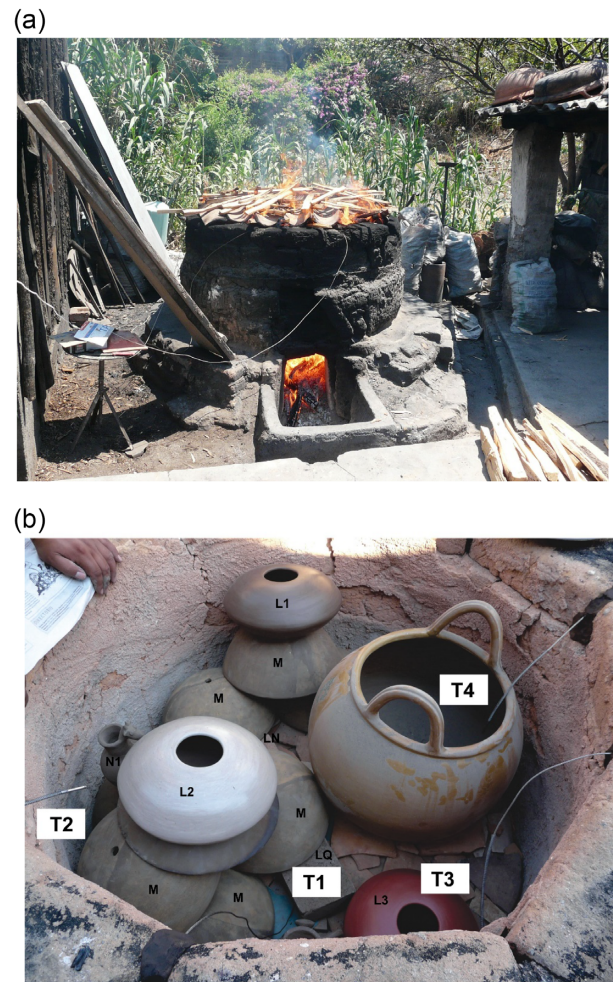
Figure 1. Baking of ceramic reproductions. (a) Picture of the kiln during the heating procedure. (b) Baking compartment of the oven with archaeological artefacts and thermocouples T1 to T4. Names of archaeological pieces are indicated.
