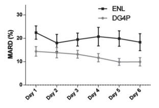
Figure 4. Average continuous glucose monitoring accuracy per day (mean absolute relative difference (MARD)  $\pm$  95% confidence interval) for the Dexcom<sup>®</sup>G4 Platinum (DG4P) and the Medtronic Paradigm Veo Enlite (ENL) systems.
