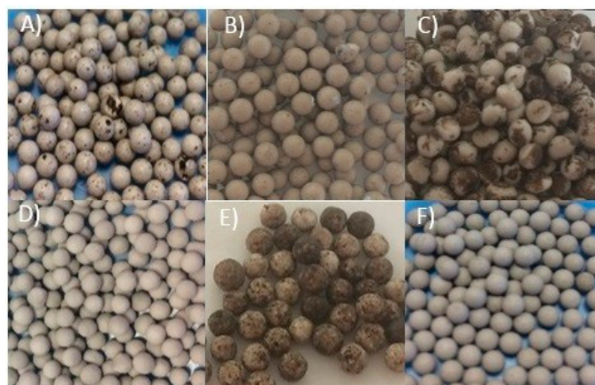
Figure 1. Appearance of the homogeneously dispersed catalysts: (A) CP-DI-Ea, (B) CP-WI-Ea, (C) RP-DI-Ec, (D) CP-DI-Ab, (E) RP-DI-Aa, and (F) RP-DI-Ab.
