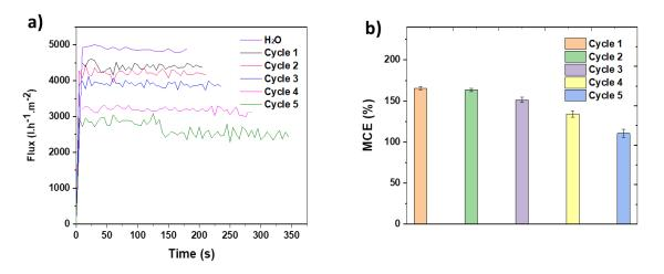
**Figure 7.** (a) Flux of H<sub>2</sub>O and treated solution as function of cycle number, b) Stability of F-rGO membrane for PCM removal using pilot plant coupling EF process and filtration.  $V_{solution} = 2.5$  L, PCM (0.1 mM), Na<sub>2</sub>SO<sub>4</sub> (50 mM), FeSO<sub>4</sub> (0.2 mM), pH = 3, I = 170 mA.
