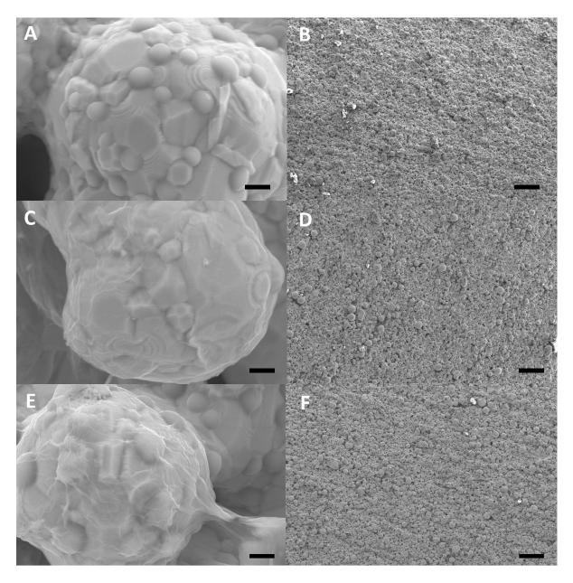
**Figure 3.** SEMs of the (A, B) bare SS membranes as well as (C, D) after GO and (E, F) rGO coating. The scale bars for A, C and E corresponds to 1 micrometer, while those of B, D and F to 100 micrometers.
