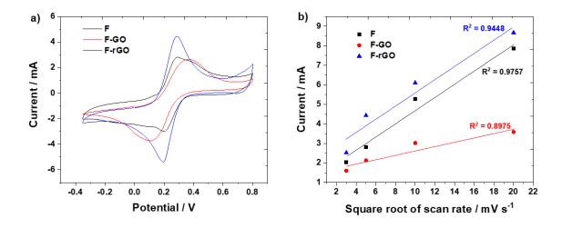
**Figure 5.** a) CV at scan rate of 5 mV s<sup>-1</sup> and (b) the relationship between peak current and scan rate ( $\sqrt{\gamma}$ ) of F, F-GO, F-rGO membranes.
