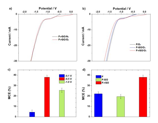
**Figure 6.** a) LSV of a) F-rGO under N<sub>2</sub>/O<sub>2</sub> atmosphere, b) F, F-GO, F-rGO cathodes obtained in 50 mM Na<sub>2</sub>SO<sub>4</sub>, O<sub>2</sub> saturated solution, pH = 3. Scan rate 5 mV/s; MCE of PCM mineralization by EF process in bath experiment at applied potential of c) -0.1 V, -0.5 V, -1.0 V using F-rGO cathode, d) -0.5 V using F, F-FO, F-rGO cathodes.
