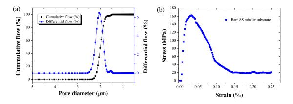
**Figure 2.** (a) Pore size distribution and (b) mechanical strength of the bare SS HF. The mean pore size of the bare membranes was calculated at 1.9  $\mu$ m +/- 0.2  $\mu$ m and the maximum flexural stress at 162 ± 15 MPa.
