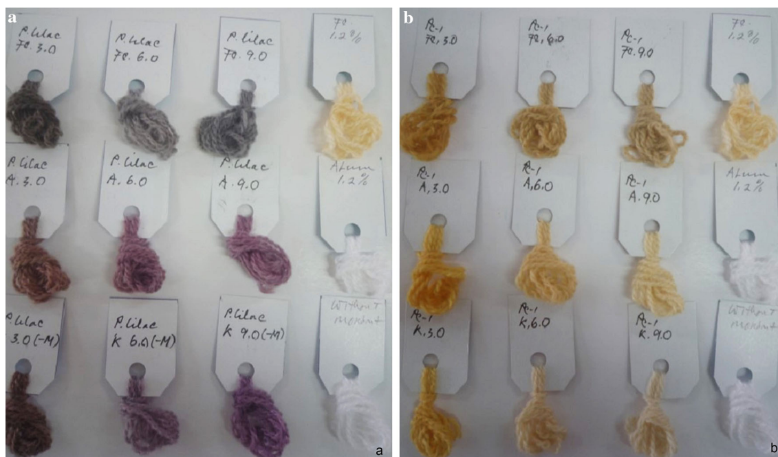
Fig. 54 a Colour variation on woolen yarn dyed with Purpureocillium lilacinum dye with different mordants and dyeing pH. b Colour variation on woolen yarn dyed with Penicillium sp. dye with different
