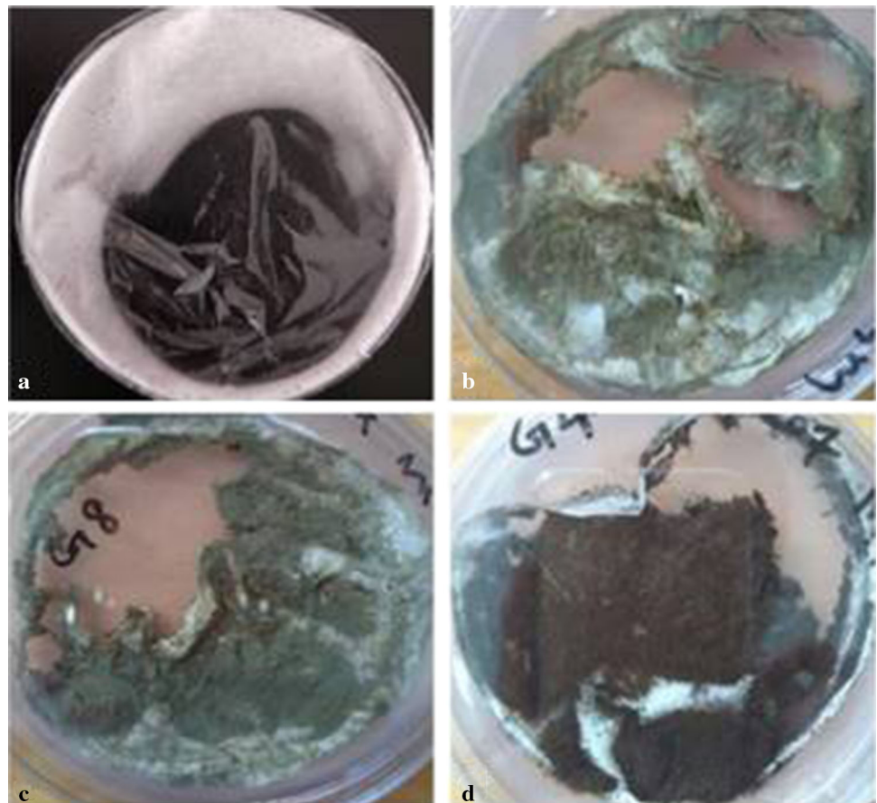
Fig. 45 Fungal degradation of polyester polyurethane (PEU) films. a PEU film not exposed to fungal degradation (control); b–d PEU films exposed to different Aspergillus spp. on malt extract agar medium incubated for 28 days in dark at 30 °C. The extent of biodegradation differed for each strain. Fungal hyphal growth is observed on the PEU surface and some portions of the PEU films are degraded due to fungal activities
