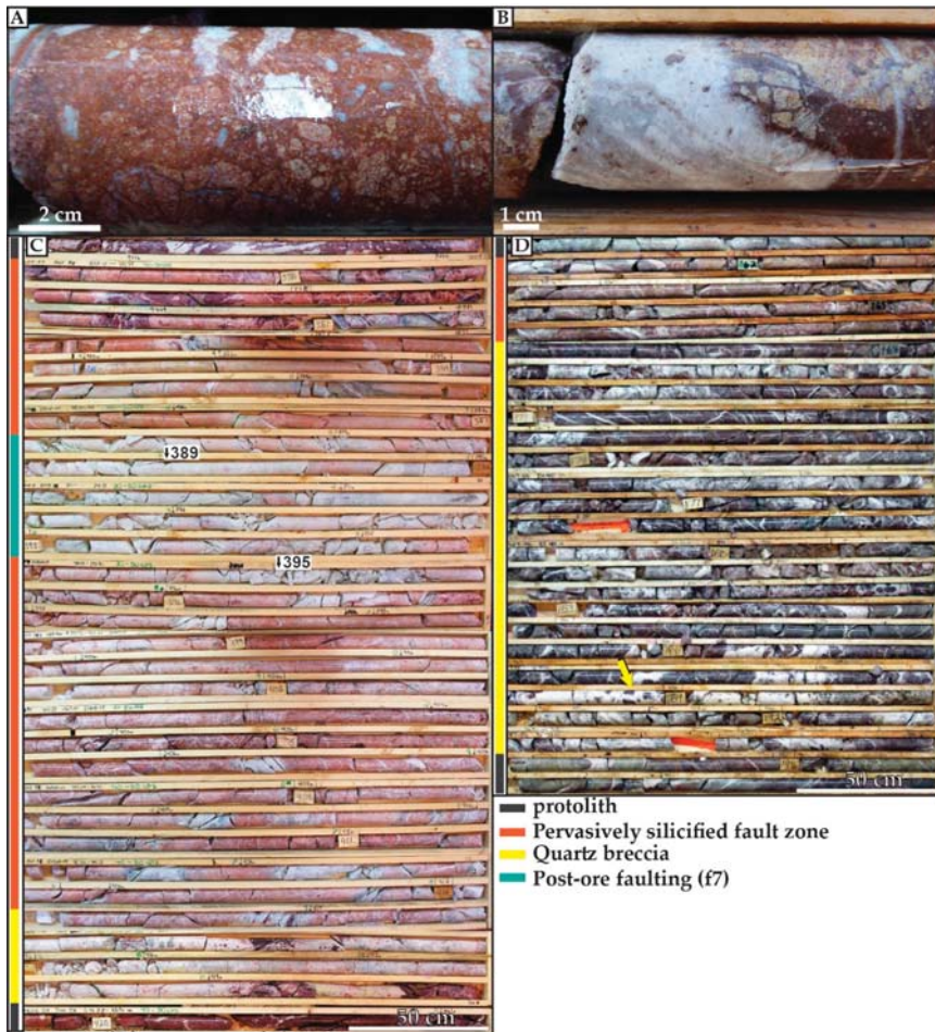
Figure 4. (A) Pervasively silicified cataclastic fault rock; (B) same as (A), crosscut by a white quartz vein of the QB; (C) pervasively silicified fault zone crosscut by late fracturing and clay alteration event (End deposit); and (D) typical intersection of the QB displaying deep purple hematized rock, massive and minor white quartz veins. Jigsaw textures are locally observable (e.g., at 189 m, yellow arrow; Contact prospect).
