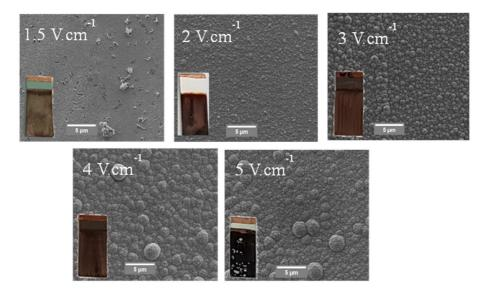
Figure 6: Top-view SEM micrographs of the obtained deposits for applied electric fields (1.5, 2, 3, 4, 5V cm<sup>-1</sup>).
