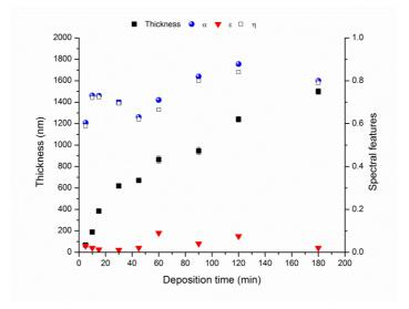
Figure 10: Calculated  $\alpha$ ,  $\varepsilon$  and  $\eta$  and measured deposit thickness as a function of deposition time (min).
