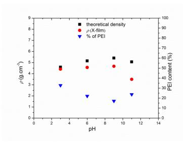
Figure 5: Variation of deposit density and %V of PEI as a function of pH
