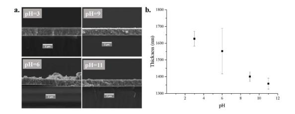
Figure 3: SEM cross-sections (a) of CuO/PEI deposits at pH= 3, 6, 9 and 11 for  $E=2V \text{ cm}^{-1}$  and t=120 min and corresponding measured thickness versus pH (b).
