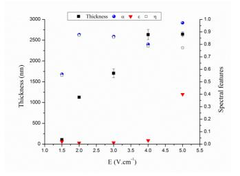
Figure 9: Measured thickness and spectral features of the obtained deposits at 1, 1.5, 2, 3, 4, 5V cm<sup>-1</sup> for deposition time of 120 min.
