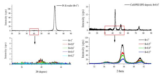
Figure 12 : GIXRD scans of (right) of Pt Si wafer and (left) of CuO/PEI EPD deposit (E=2 V.cm<sup>-1</sup>, t=120 mins).
