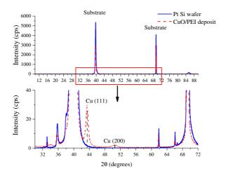
Figure 11: 0/20 scan of XRD spectra of Pt Si wafer and CuO/PEI deposit.
