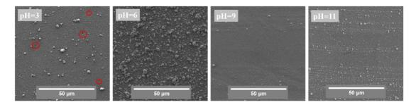
Figure 4: Top-view SEM micrographs of EPD deposit of CuO/PEI obtained at pH=3. Holes generated from electrolysis reaction are shown in red.
