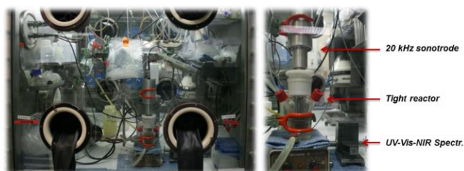
Fig. 2. This experimental setup was used to perform 20-kHz sonochemical experiments at the Atalante facility in Marcoule. This device consists of a tight reactor that can control temperature, a circulation of carrier gases, and even the sampling of solution during sonolyses. The cell is cooled from outside the box and an UV-Vis-NIR spectrophotometer is also connected to the enclosure.
