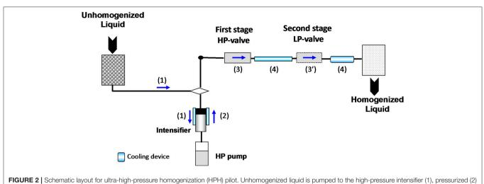
and forced through high pressure (HP) then low-pressure (LP) valves (3-3'). Fluid temperature heating is limited by cooling devices (4).
