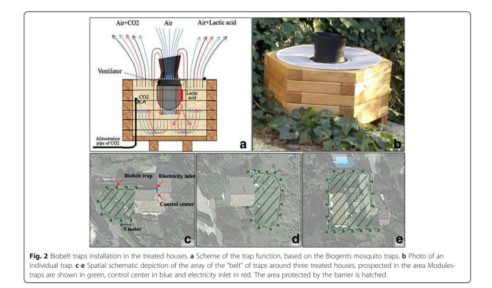
system was made of several elements: the traps, the electrical system and  $CO_2$  connections, the programming unit, a 12 V transformer, and  $CO_2$  bottles. Twelve, 16 and 23 h of a technicians work time were devoted to the installation of the system. Around 630 h of emission of  $CO_2$  per house were used during this study, yielding a total of 6.3 kg of  $CO_2$  per trap, and as a result 56.7, 81.9 and 113.4 kg of  $CO_2$  for each house, respectively.
