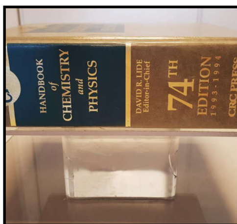
Figure 5. A 25 \times 20 \times 20 \text{ cm}^3 -hydrogel block overlaid by a 3.2 kg weight (corresponding pressure of 10^{-3} \text{ MPa} ).
