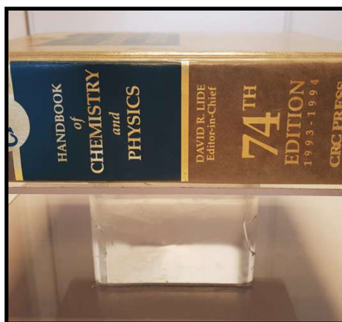
Figure 5. A 25 \times 20 \times 20 cm 3 -hydrogel block overlaid by a 3.2 kg weight (corresponding pressure of 10^{-3} MPa).
