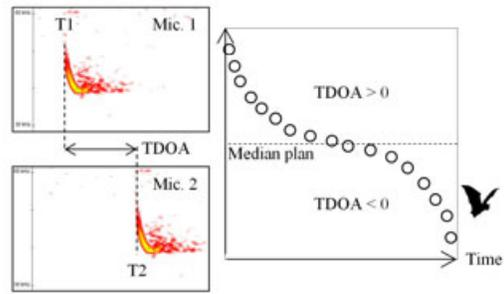
**C** Definition of a bat road crossing event with a pair of acoustic recorders
