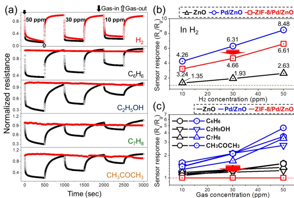
**Figure 6.** (a) Dynamic normalized resistance curves of Pd/ZnO and ZIF-8/Pd/ZnO NWs gas sensors to 10, 30 and 50 ppm H<sub>2</sub>, C<sub>6</sub>H<sub>6</sub>, C<sub>2</sub>H<sub>5</sub>OH, C<sub>7</sub>H<sub>8</sub> and CH<sub>3</sub>COCH<sub>3</sub> gases. (b) Calibration curves of bare ZnO,
