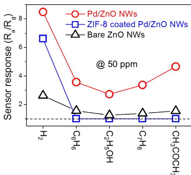
**Figure 7.** Sensing responses of bare ZnO NWs, Pd/ZnO NWs and ZIF-8 coated Pd/ZnO NWs gas sensors to 50 ppm of H<sub>2</sub>, C<sub>6</sub>H<sub>6</sub>, C<sub>7</sub>H<sub>8</sub>, C<sub>2</sub>H<sub>5</sub>OH and CH<sub>3</sub>COCH<sub>3</sub> gases in air at 200°C.
