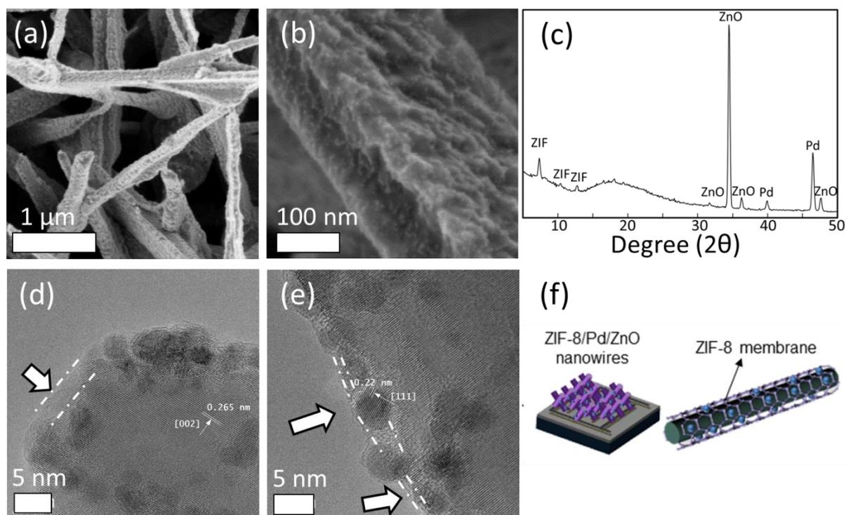
**Figure 4.** (a,b) SEM images of ZIF-8/Pd/ZnO NWs, (c) GI-XRD diffraction patterns (the ZIF-8, ZnO and Pd peaks are indicated), and (d,e) HRTEM images of the ZIF-8/Pd/ZnO NWs sensing nanomaterial (the
