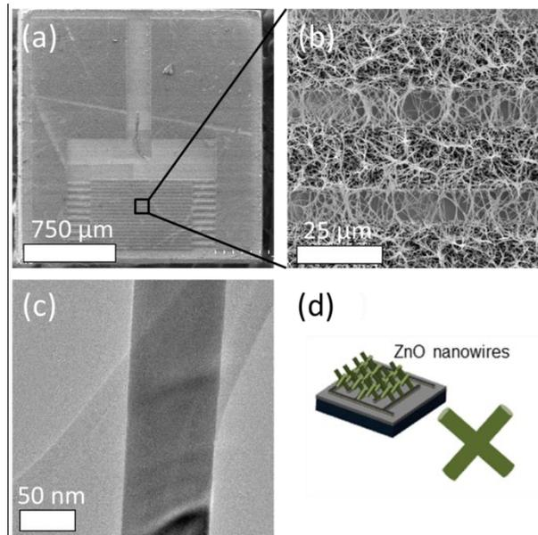
**Figure 2.** (a,b) SEM images of the entire sensor device and a zoom for visualizing interconnected ZnO NWs on the sensor surface, (c) TEM image of a single ZnO NW, and (d) schematic representation of the bare ZnO NWs sensor.
