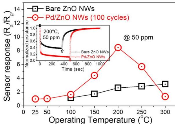
**Figure 5.** Sensor responses of bare ZnO and Pd/ZnO gas sensors to 50 ppm H<sub>2</sub> gas, as a function of sensing temperature. Inset shows the normalized dynamic resistance curves of bare ZnO and Pd/ZnO gas sensors to 50 ppm H<sub>2</sub> gas at optimal sensing temperature (200°C).
