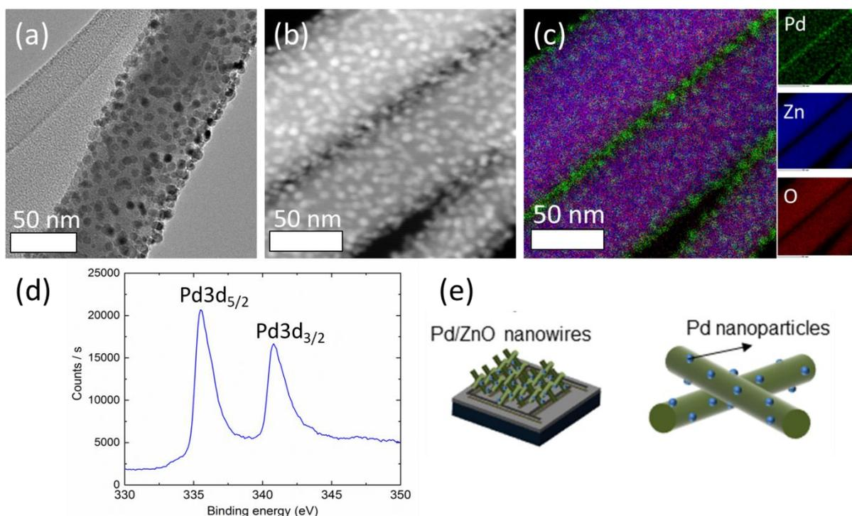
**Figure 3.** (a) TEM image of a single NW revealing a high dispersion of NPs. (b) SEM image of three NWs decorated with Pd NPs and (c) corresponding EDX mapping. (d) XPS spectra of the Pd 3d scan of the ZnO NWs decorated with Pd NPs. (e) Schematic representation of the Pd/ZnO NWs sensor.
