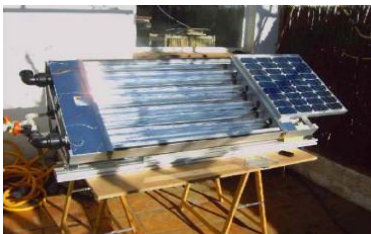
Figure 22: Autonomous solar prototype of water purification of European projects AQUACAT and SOLWATER 338 .
