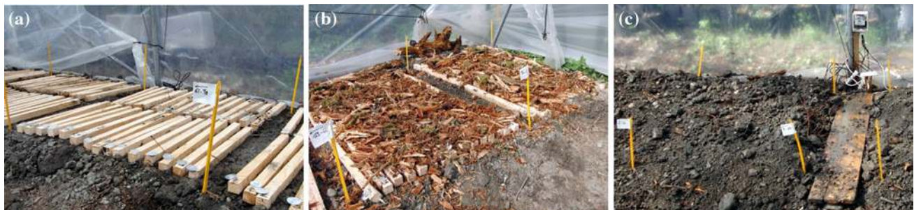
Fig. 1 Successive steps of sample installation in the greenhouse. a Intact samples divided into series; b samples covered with the first layer of woody debris; c samples covered by the second layer of soil
