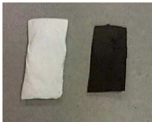
Figure 1. Images of the PAN fibers mat (white) and CNFs mat (black).
