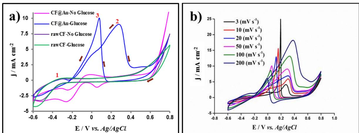
**Figure 5.** Cyclic voltammograms in  $10 \text{ mM}$  glucose in  $0.1 \text{ M}$  KOH of (a) Au@CF and raw CF anodes in the presence and absence of  $10 \text{ mM}$  glucose at  $50 \text{ mV s}^{-1}$ , and of (b) Au@CF anode at various scan rates.
