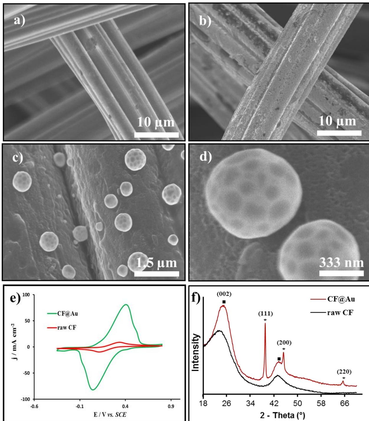
**Figure 1.** SEM images of (a) raw CF, (b) Au@CF without thermal treatment, (c, d) Au@CF after heating treatment at 1000  $^{\circ}\text{C}$  for 1h, (e) Cyclic voltammograms of raw CF and Au@CF electrodes in potassium hexacyanoferrate solution
