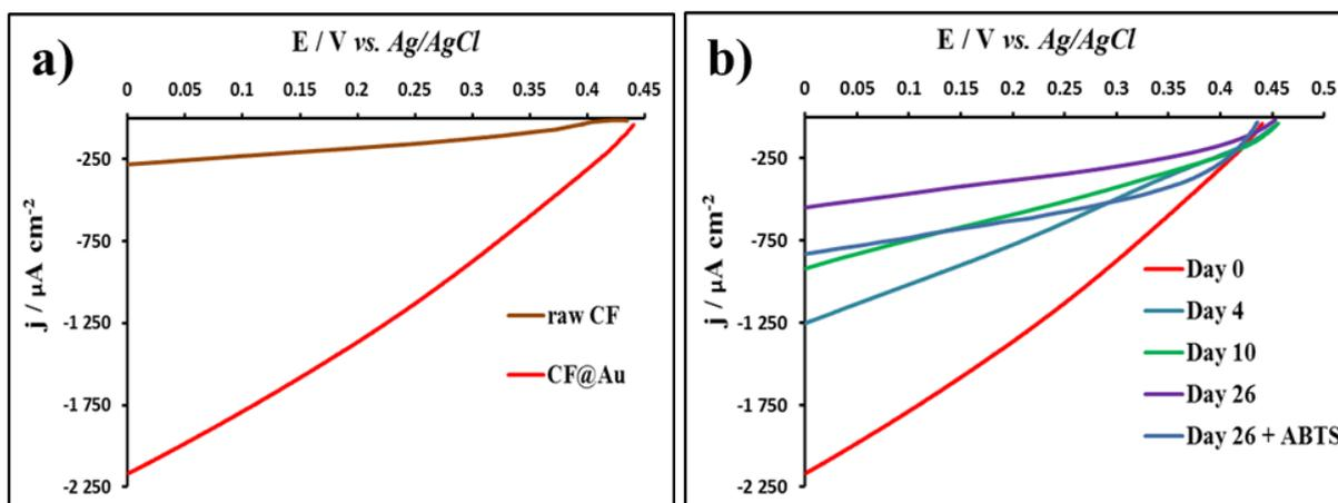
**Figure 4.** (a) Polarization curves of O<sub>2</sub> electroreduction on the Au@CF and the raw CF biocathodes modified with the enzyme BOD. (b) Stability of the BOD-immobilized Au@CF electrode with time. Scan rate of 3 mV s<sup>-1</sup>, O<sub>2</sub>-saturated PBS 0.1 M, pH 7.0 at 30 °C.
