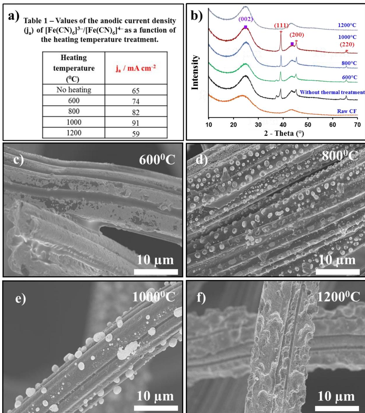
**Figure 3.** (a) Table 1 – Values of the anodic current density ( $j_a$ ) of  $[\text{Fe}(\text{CN})_6]^{3-}/[\text{Fe}(\text{CN})_6]^{4-}$  as a function of the heating temperature treatment. (b) X-ray diffraction patterns of Au@CF ( $0.05 \text{ mg mL}^{-1}$   $\text{HAuCl}_4 \cdot 3\text{H}_2\text{O}$ ) electrodes at different
