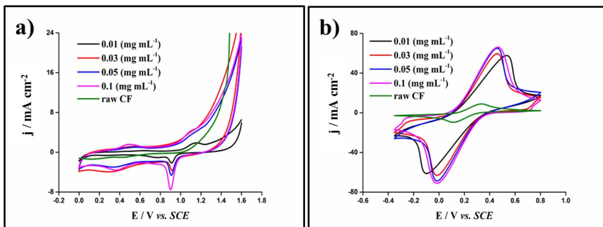
**Figure 2.** Cyclic voltammograms of raw CF and Au@CF electrodes (projected surface area of  $1 \text{ cm}^2$ ) at different chloroauric acid trihydrate concentrations in (a)  $0.5 \text{ M H}_2\text{SO}_4$ , and (b) potassium hexacyanoferrate solution ( $10 \text{ mM}$ ) in  $1 \text{ M KNO}_3$ . Scan rate  $10 \text{ mV s}^{-1}$ .
