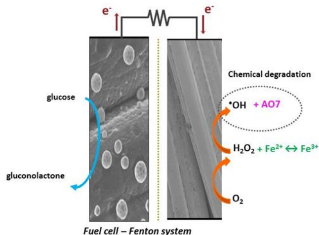
Figure 5-9. Schematic diagram of the Fuel Cell-Fenton system. Reprinted from Ref. [110]. Copyright (2016), with permission from RSC Publishing .
