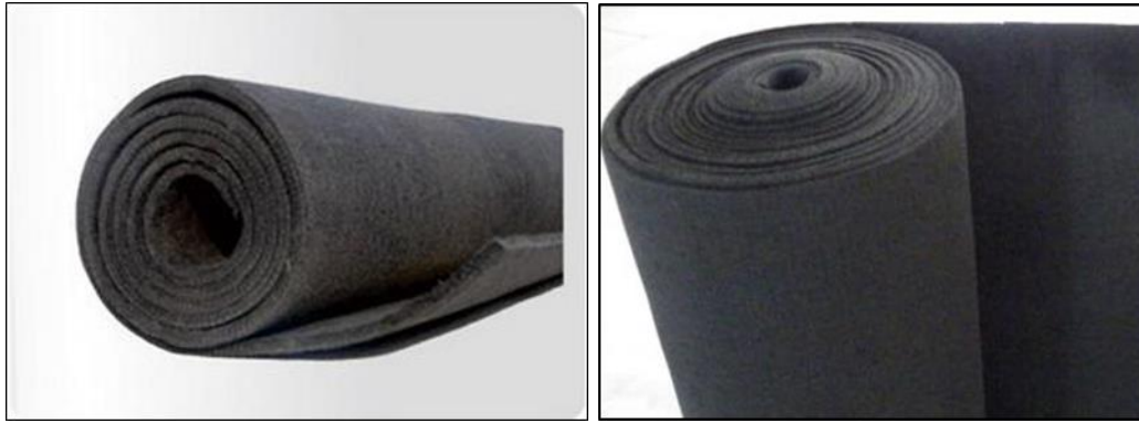
Figure 2-2. Typical shape of commercial (a) CF and (b) GF. (Product information from CeraMaterials ( http://www.ceramaterials.com/graphitecarbonfelt.html . Updated 04/2017)).
