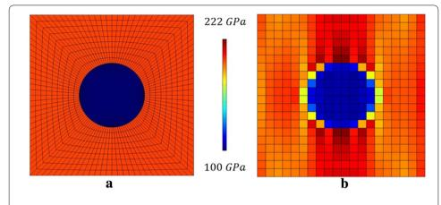
**Fig. 3** Identified Young modulus distributions: **a** 2 "consistent" identification domains and **b** 400 non-consistent identification domains
