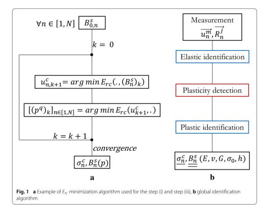
As already mentioned, we focus on a J2 elastoplastic model with kinematic hardening and no more than three material constants can be locally identified at each load step. The identification algorithm involves three steps (see Fig. 1b): (i) an elastic identification, (ii) a plasticity detection and (iii) a plastic identification.
