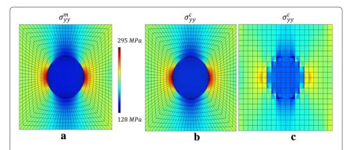
**Fig. 4** Distribution of transversal stress fields: **a** "measured" stress field  $\sigma_{yy}^m$  (from FE simulation), **b** identified stress field  $\sigma_{yy}^c$  using 2 "consistent" identification domains and **c** identified stress field  $\sigma_{yy}^c$  using 400 non-consistent identification domains
