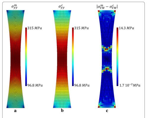
**Fig. 6** Distribution of transversal stress fields:  $\mathbf{a} \, \sigma_{yy}^m$  from a FE simulation,  $\mathbf{b} \, \sigma_{yy}^c$  the identified and  $\mathbf{c}$  von Mises norm of the absolute error on stress
