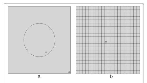
**Fig. 2** Geometry for the identification: **a** two identification domains respecting the material heterogeneity and **b** 400 identification domains that do not respect the material heterogeneity
