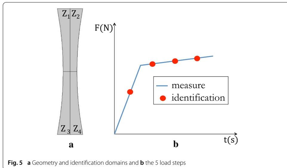
**Fig. 5** **a** Geometry and identification domains and **b** the 5 load steps
