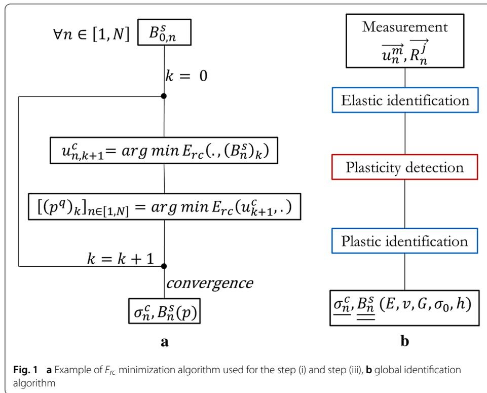
As already mentioned, we focus on a J2 elastoplastic model with kinematic hardening and no more than three material constants can be locally identified at each load step. The identification algorithm involves three steps (see Fig. 1b): (i) an elastic identification, (ii) a plasticity detection and (iii) a plastic identification.
