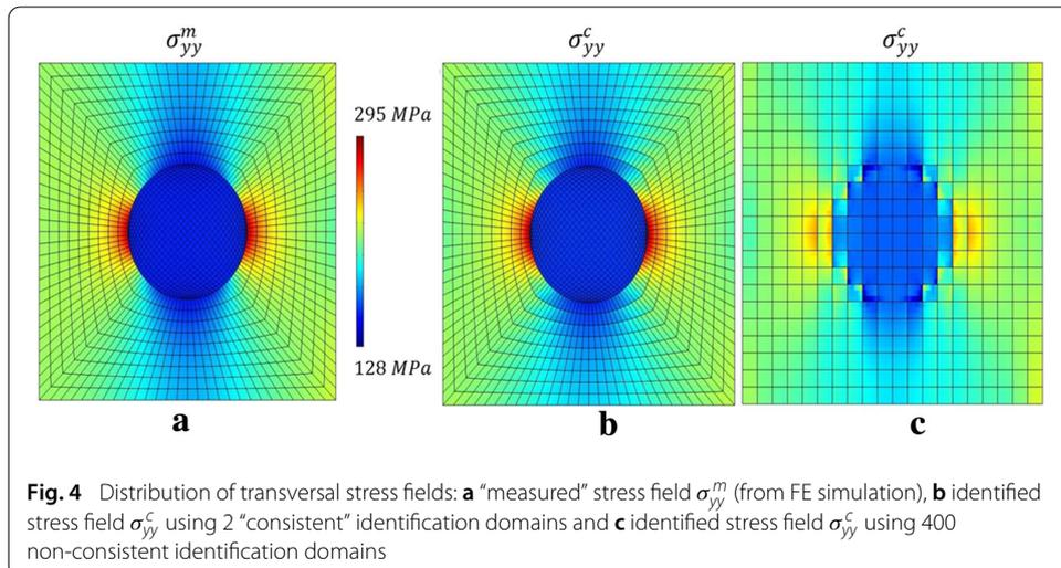
Figure 4b shows that the identified stress fields are very close to the reference values. The maximum error is about 4% of the maximum stress (295 MPa) and is located in the zones of maximum stress gradient.
