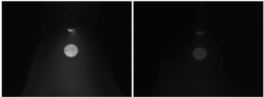
figure, it is observed low plasma emission at these wavelengths. In the left figure, the liquid at the wire tip is visible. This leads to a punctual reflection at the top of the droplet that can modify locally the temperature measurement.
